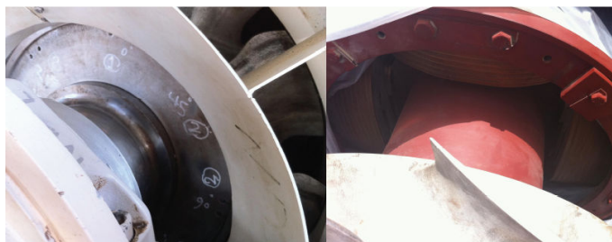
Fig. 29 Balancing weights positions (dynamic balancing panel-panel 2)
