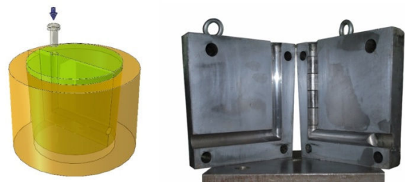
Fig. 2 ECAP die set-up used in this research
