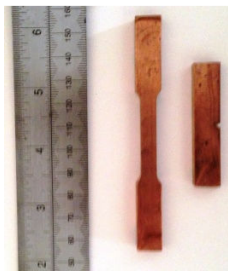
Fig. 4 Tensile and impact test specimens
