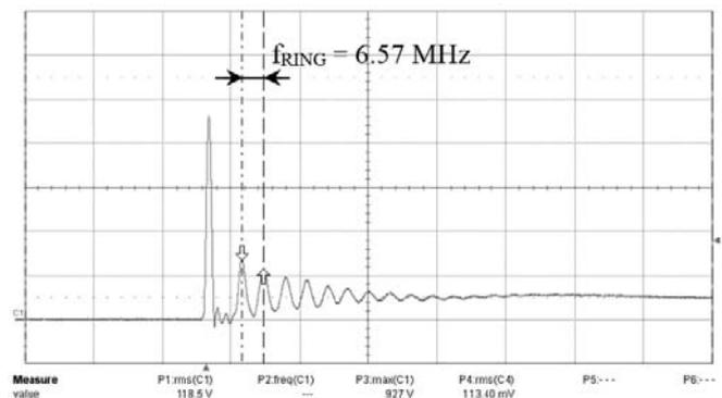
Fig. 12 The detail of ringing transistor  $V_{DS}$  voltage peak during switching-off (200 V/div, 500 ns/div,  $V_{pp} = 927$  V)
