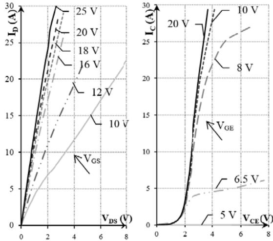
Fig. 2 Measured static characteristics  $I_D = f(V_{DS})$  of SiC MOSFET transistor (left) and of Si IGBT  $I_C = f(V_{CE})$  (right)
