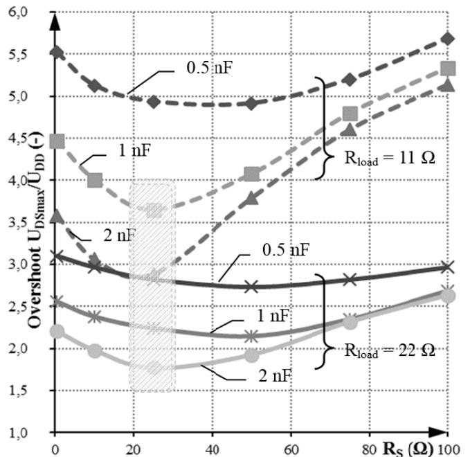
Fig. 14 The graph of voltage overshoot  $U_{DSmax}/U_{DD}$  (-) with different value  $R_S$ ,  $C_S$  and for load resistor  $11 \Omega$  (8 A) and  $22 \Omega$  (13 A)
