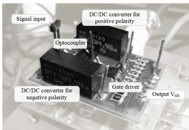
Fig. 7 Realized SiC MOSFET driver with test points
