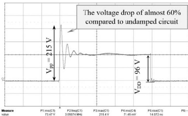
Fig. 16 The transistor voltage  $V_{DS}$  with RC snubber  $C_S = 1 \text{ nF}$ ,  $R_S = 25 \Omega$  (100V/div, 1μs/div)
