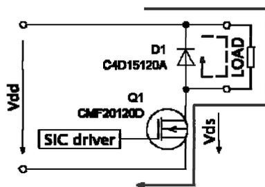
Fig. 10 Buck converter and direction of current
