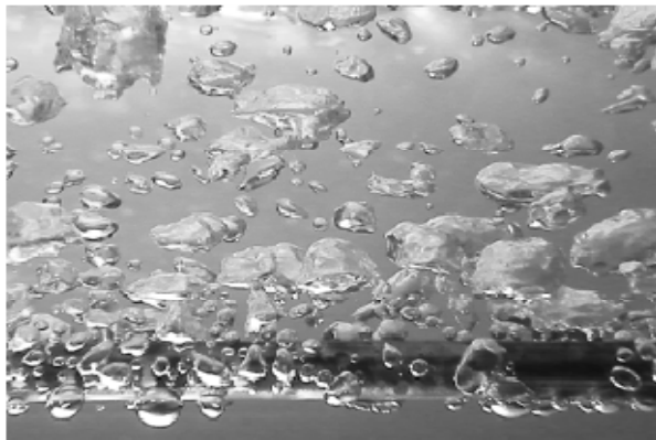
Fig. 3 Pool boiling of pure water under heat flux of 60 Kw/M 2
