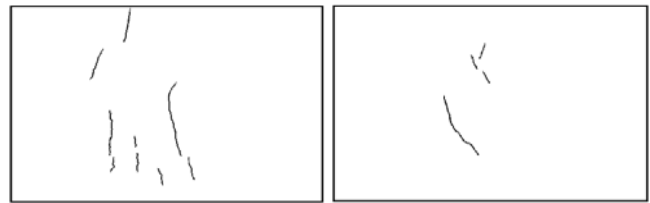
Fig. 10 Plastic shrinkage cracking 1.50% RP fiber, length 20mm
