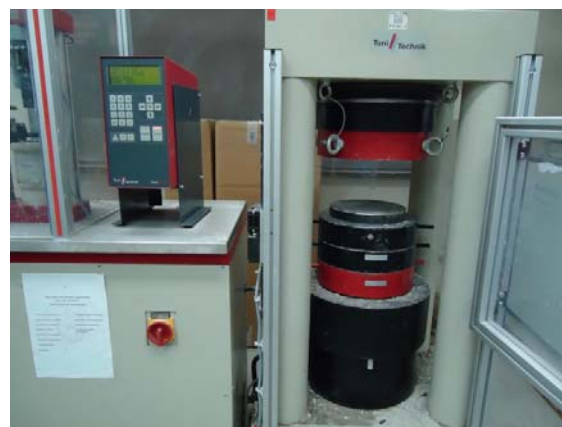
Fig. 4 Compressive strength testing machine
