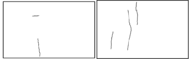
Fig. 8 Plastic shrinkage cracking 0.50% RP fiber, length 20mm
