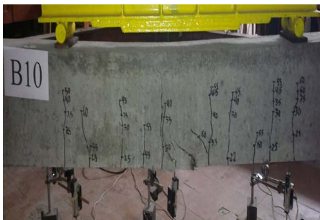
Fig. 6 Typical splitting failure for beam specimens with confining transverse reinforcement in splice region
