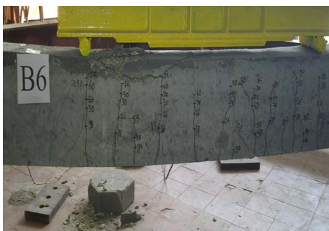
Fig. 7 Typical flexure failure for beam specimens
