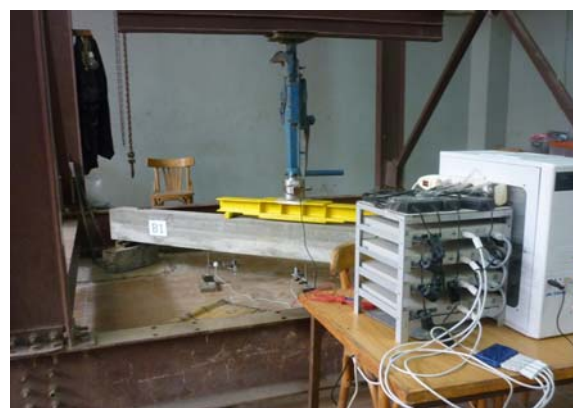
Fig. 4 Splice beam prior to testing
