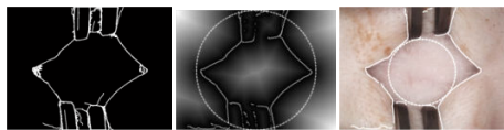
Fig. 8 (Left to right) An edge map, a distance map overlaid with the edge map and a circular region of interest, and the fitted circle
