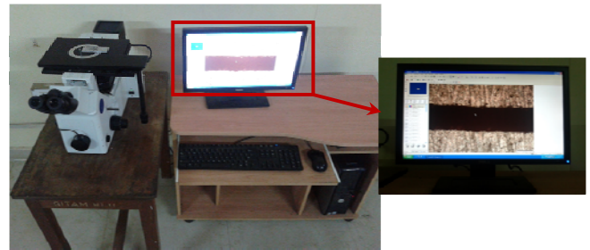
Fig. 1 Experimental setup for kerf measurement
