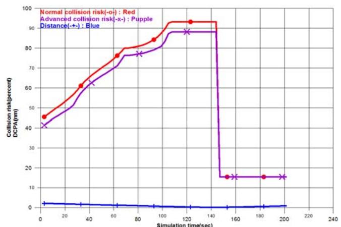
Fig. 11 The collision risk and distance –non-collision situation
