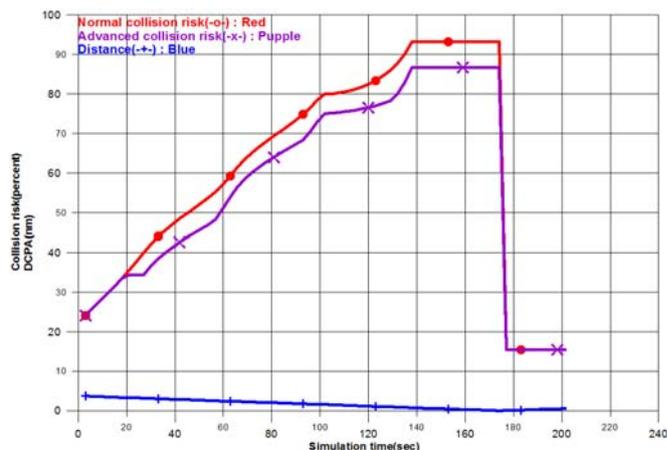
Fig. 7 The collision risk and distance – non-collision situation
