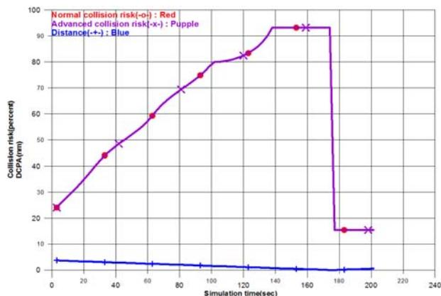
Fig. 5 The collision risk and distance – collision situation
