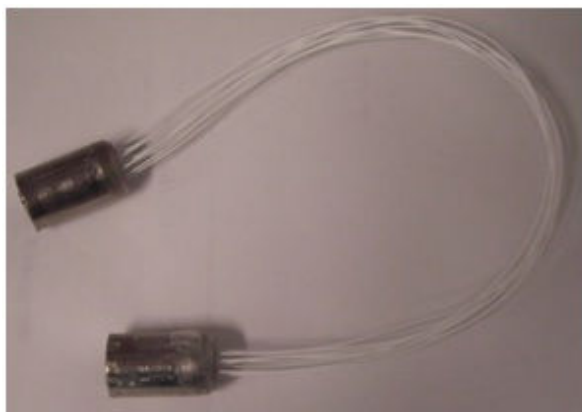
Fig. 1 Polypropylene hollow-fibre membranes set in membrane fittings
