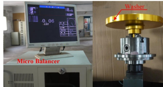
Fig. 13 Wafer carrier and dynamic balancing
