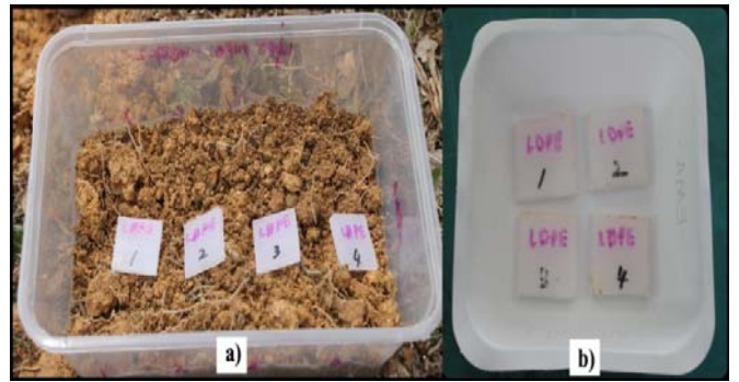
Fig. 6 Sample of pure LDPE a) before and b) after the soil burial test
