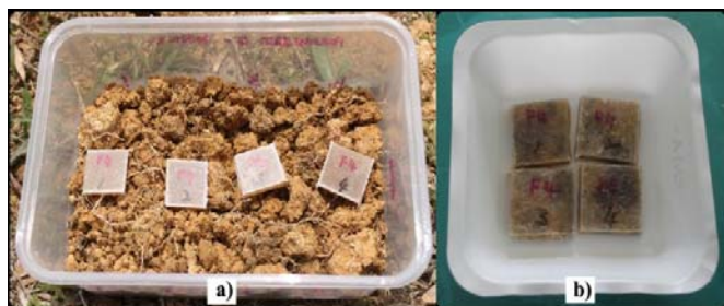
Fig. 10 Sample of LDPE/TS: 40/60 a) before and b) after the soil burial test
