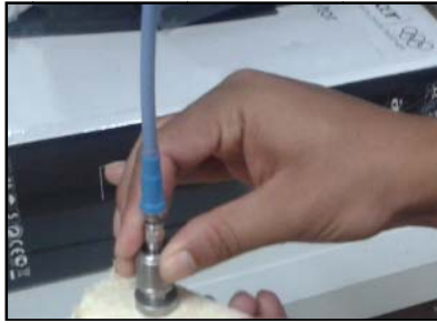
Fig. 3 Defining dielectric properties using dielectric probe
