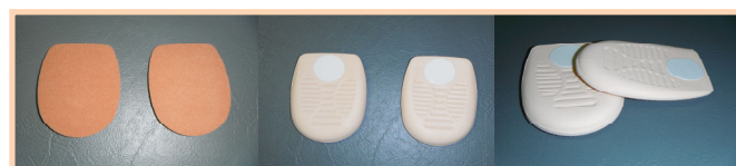
Fig. 8 Specimen 2 (natural latex foam)
