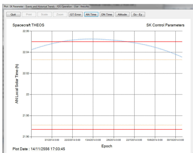
Fig. 4 Drift in local solar time of the ascending node prediction
