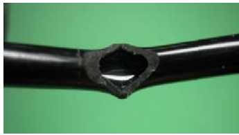
Fig. 2 Deformation of the CSDS during bending
