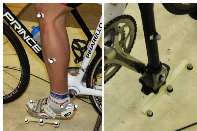
Fig. 3 Reflective markers on health limb (left), on prosthesis (right)
