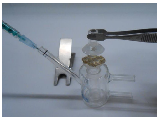
Fig. 1 Photograph of Franz Diffusion cell with a shed snake skin in between the donor and receptor parts
