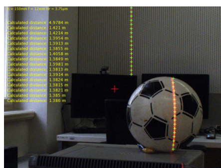
Fig. 10 Distance measurement on spherical object
