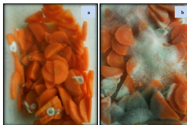
Fig. 11 Photographic images for (a) sample stored in nano-silver container packaging (b) control stored conventional container packaging, at 35°C for 7 days
