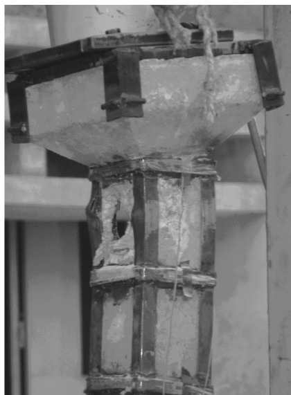
Fig. 20 Failure mode of eccentrically loaded strengthened column
