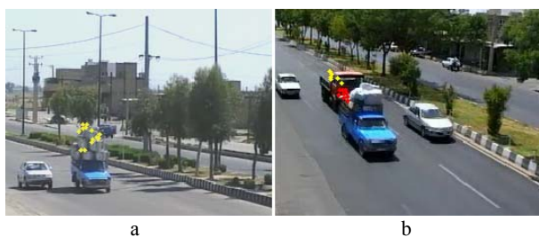
Fig. 6 a. Result of second test, an over-height vehicle detection (over 2.5 meters) b. Result of third test, an over-height (2.5 meter) detection in occlusion situation
