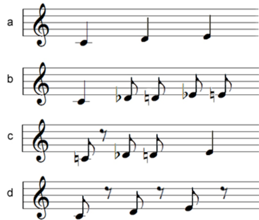
Fig. 11 (a) original played notes with electronic keyboard, (b),(c) transcribed notes in none silent environment, (d) transcribed notes when used some filters in hardware power supply and isolated analog and digital units
