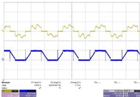
Fig. 9 Phase current and phase voltage waveform
