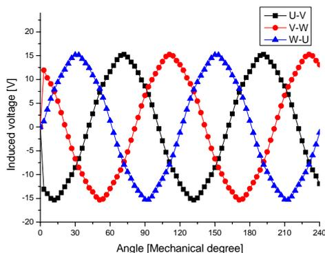
Fig. 2 Calculated back EMF waveform @ 10,000rpm
