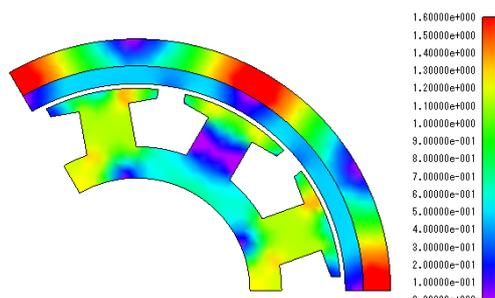
Fig. 1 Flux line and density distribution
