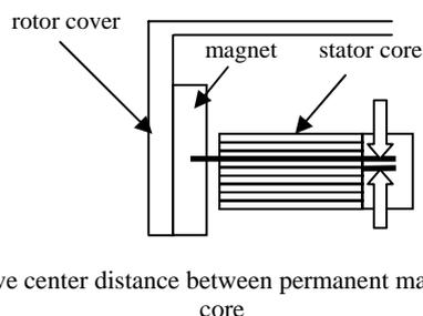
Fig. 3 Relative center distance between permanent magnet and stator core
