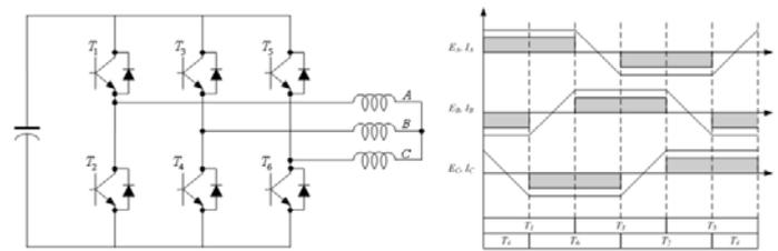
Fig. 6 Inverter configuration and current commutation sequence for BLDC
