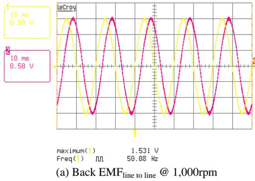
(a) Back EMF<sub>line to line</sub> @ 1,000rpm
