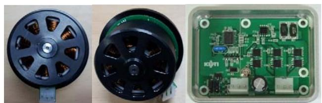
(a) BLDC motor and separate drive
