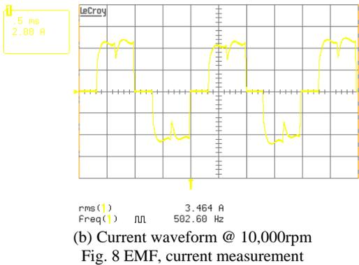
(b) Current waveform @ 10,000rpm
