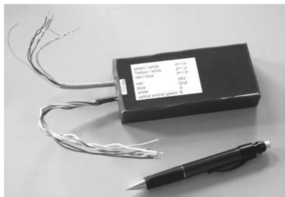
Fig. 1 The magnetic detector is within its housing. Various housing shape can be applied to fit different detector locations and applications
