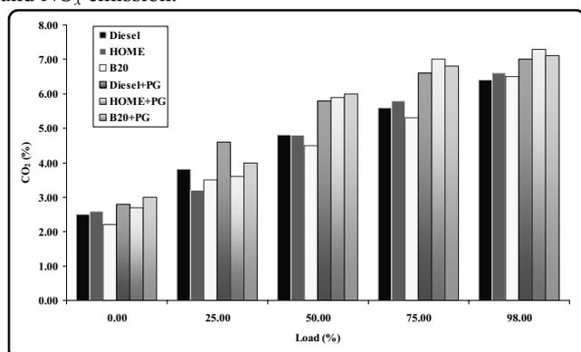
Fig. 6 Variation of CO<sub>2</sub> emission with applied load in liquid fuel and dual fuel mode
