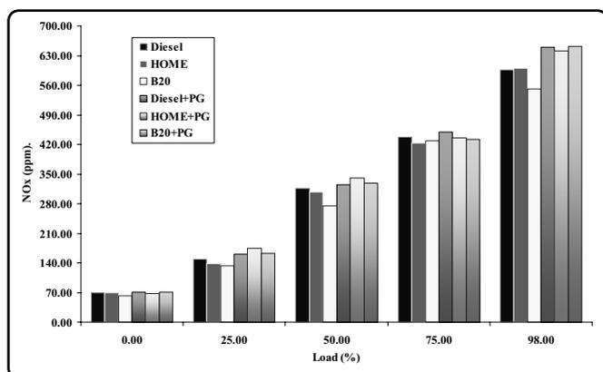
Fig. 7 Variation of NO<sub>x</sub> emission with applied load in liquid fuel and dual fuel mode
