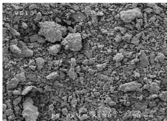
Fig. 13 FE-SEM image of Al-CNT composite after sonication
