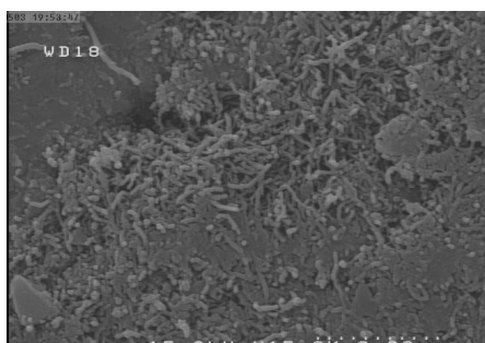
Fig. 17 FE-SEM image of Al-CNT composite after compaction
