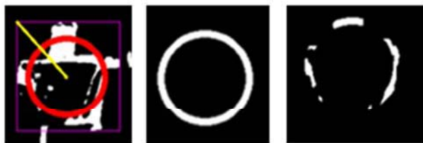
Fig. 13 Input skins binary(Left), Circle mask(centre), and operation result(Right)
