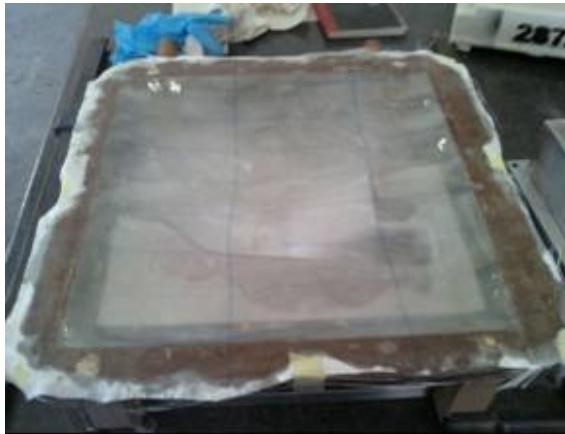
Fig. 2 Impregnated fabric with less restrain on the mould.
