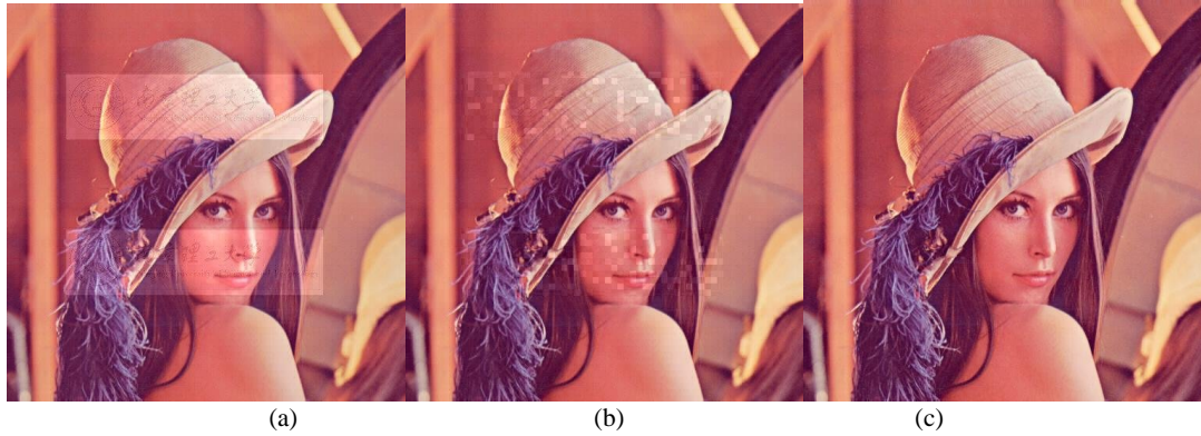
Fig. 4 Results for a = 0.2 , c = 0.3 and d = 0.5 : (a) Watermarked Image (Psnr: 17.4), (b) Remove without Right Key (Psnr: 27.3), (c) Remove with Right Key (Psnr:58.7)
