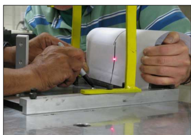
Fig. 1 Laser beam adjustment with collimator device
