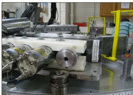
Fig. 2 Arrangement of laser beam system through adjustment with other detectors of tomography unit
