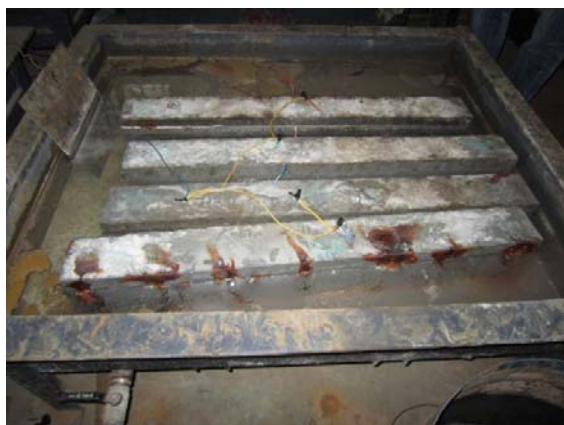
Fig. 3 Accelerated Corrosion Process for Unstressed Condition
