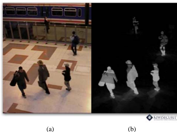
Fig. 1 A frame (a) and the corresponding background-differenced frame (b)
