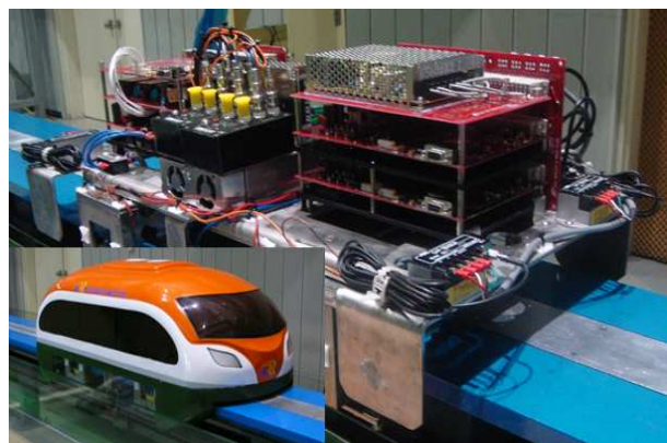
Fig. 9 The miniature maglev using hybrid magnets
