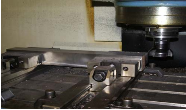
Fig. 2 The set-up for dry and wet milling testes
