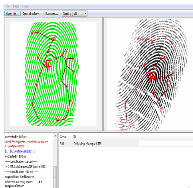
Fig. 2. An example post-matching fusion of scores (multiple samples)
