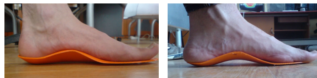
Fig. 9. Study of real compatibility between the plantar surfaces and the corrective insoles manufactured by rapid prototyping (flat foot-left, hollow foot-right)
