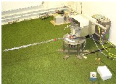
Fig. 1 The laboratory-scale single-link flexible manipulator
