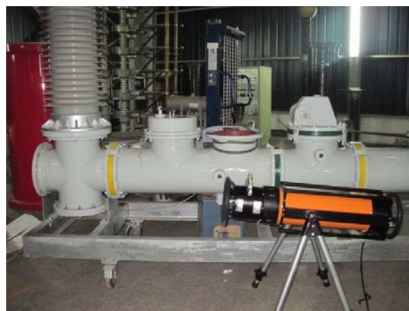
Fig. 5 X-ray machine and the imaging plate
