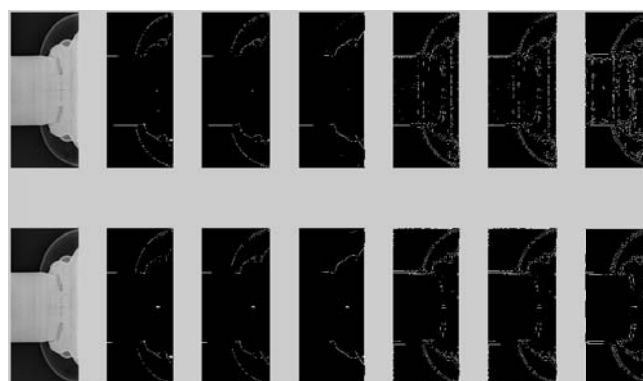
Fig. 11 the edge detection based on before and after wavelet de-noising of not fully closing position 2
