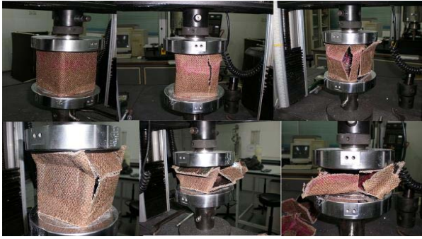
Fig. 8 Progress of Crashing Test of SQJFT
