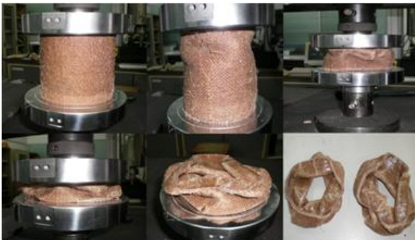
Fig. 9 Progress of Crashing Test of CJFT
