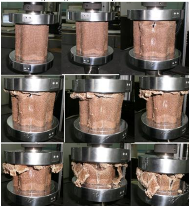
Fig.10 Progress of Crashing Test of RCJFT
