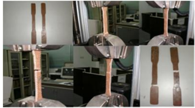
Fig. 6 Set Up of Tensile Test
