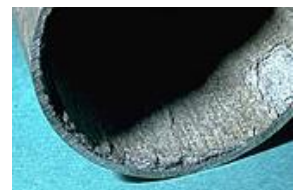
Fig. 17 Different cases of internal corrosion in metallic water pipes
