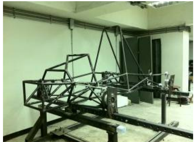
Fig. 20 Rapidamente's torsional stiffness test rig
