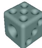
Fig. 2 The difference blend of a cube from twenty-one spheres
