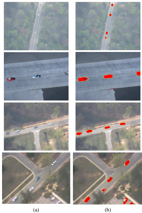
Fig. 5 Detection results of different scenes with various camera heights and angles: (a) Original image frames (b) Detected vehicles
