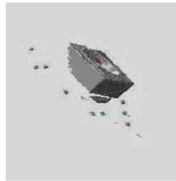
Fig. 5 An example of cloud points made by scan of insert
