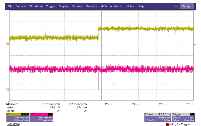
Fig. 7 The output of S&H (top), the input current to the converter (bottom)
