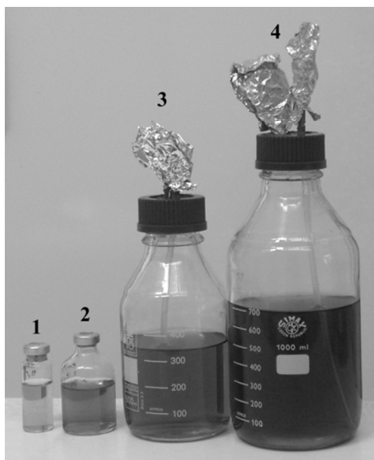
Fig. 1 The prototype scale-up experiments. (1,2) Images of air-tight serum bottles. (3,4) Images of air-tight laboratory bottles with aspiration system
