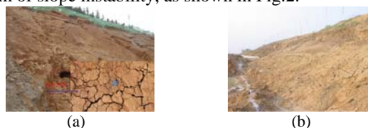
(a) Fractures of laterite (b) Shallow layer Landslide due to the dry-wet circulation Fig. 2 Common problems of fracturing laterite
