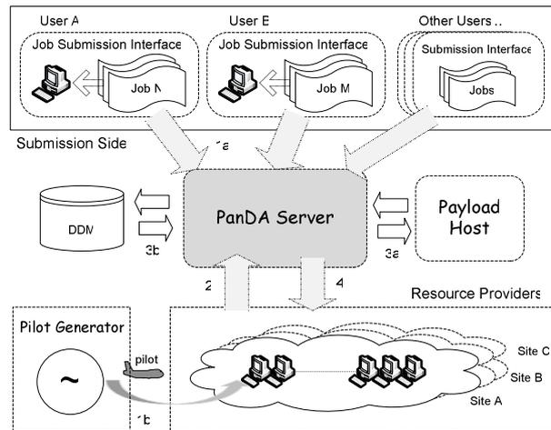
Fig. 1 High-level view of the PanDA architecture
