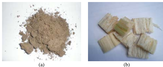
Fig. 1 The agricultural residue biofilter media (a) manure fertilizer (b) bagasse
